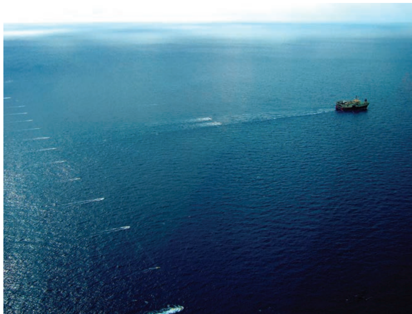
Figure 1. Seismic vessels tow air guns and multi-streamer arrays to collect seismic data. (Reproduced with permission. © Petroleum Geo-Services, Inc, 2016.)
