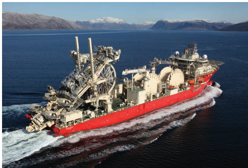
Figure 12. Flowlines and smaller pipelines are lowered to the seabed using reeled pipelay vessels. (Reproduced with permission. © Technip, 2016.)
