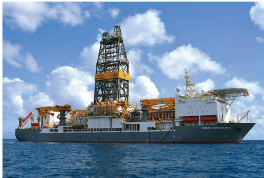
Figure 8. New drillsips can carry dual towers, two BOPs, and additional workspace as standard equipment. (Reproduced with permission. © Rowan Companies.)
