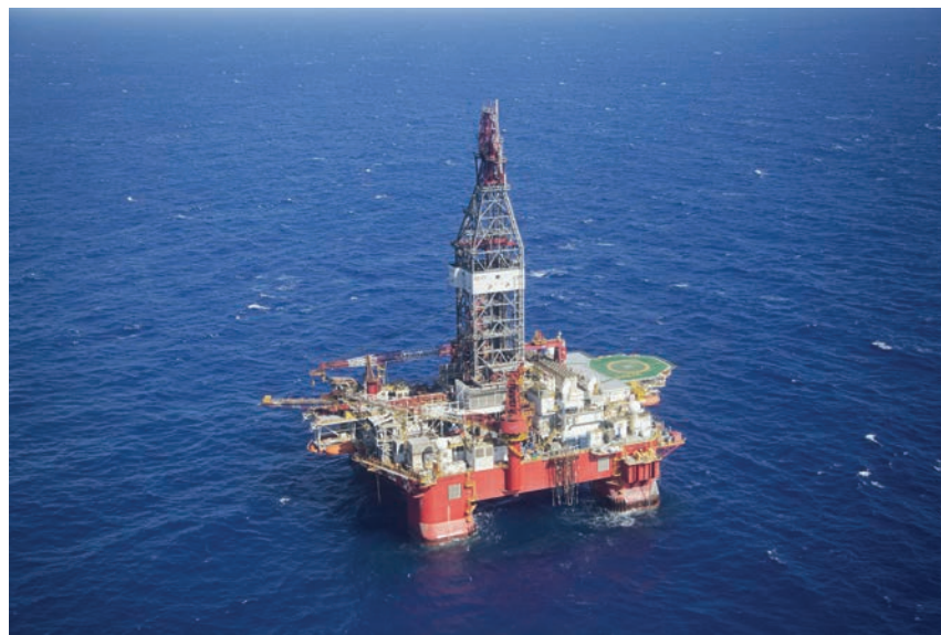
Figure 7. Modern high-specification semisubmersible rigs can drill in 12,000 feet or more of water to depths of 40,000 feet into the earth. (Reproduced with permission. © Diamond Offshore, 2016.)
