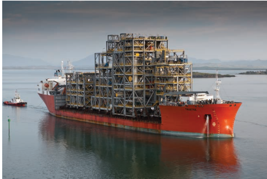
Figure 11. The offshore oil and gas industry uses many specialty vessels, such as this heavy lift vessel, for moving production modules, rigs, and other major equipment to offshore locations. (Reproduced with permission. © Dockwise, 2016.)
